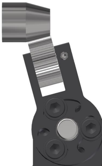
Figure 2: Good Only Suitable for pitch change less than 20%
